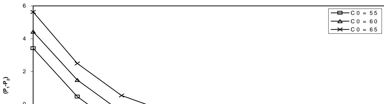
DIFFERENCE OF PROFIT ( P_1 - P_2 ) vs. FAILURE RATE ( \alpha ) FOR DIFFERENT VALUES OF THE REVENUE PER UNIT UP TIME ( C_0 )
